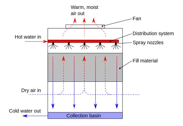
In a counterflow design, the air flow is directly opposite to the water flow (see diagram at left). Air flow first enters an open area beneath the fill media, and is then drawn up vertically. The water is sprayed through pressurized nozzles near the top of the tower, and then flows downward through the fill, opposite to the air flow.
